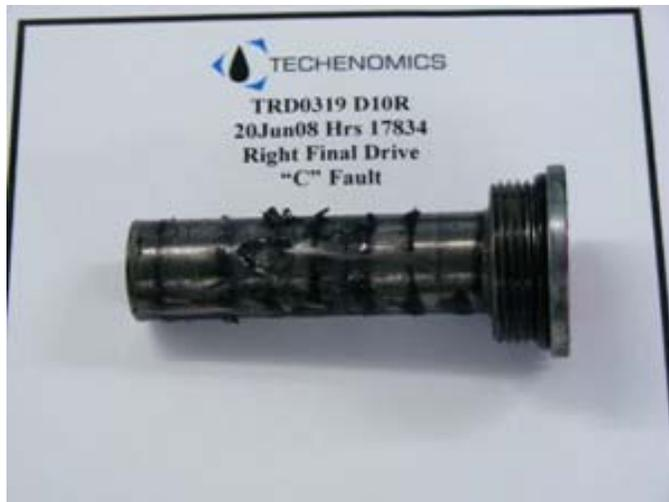
**PROBLEM:** The service interval extension to 330 hrs for all the components was achieved except for the final drives. The fleet was still experiencing unscheduled failures due to ferrous metal generation from the gears causing premature wear to the duo cone seals and gear components.
