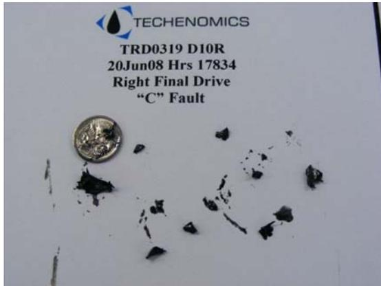
**RESULTS:** The OEI plug rods collected substantial more ferrous debris than the OEM plug rods. The debris was analyzed and potential failure areas were identified. This could not be done with the existing plugs as they did not capture debris in the similar volumes or in first wear condition.
