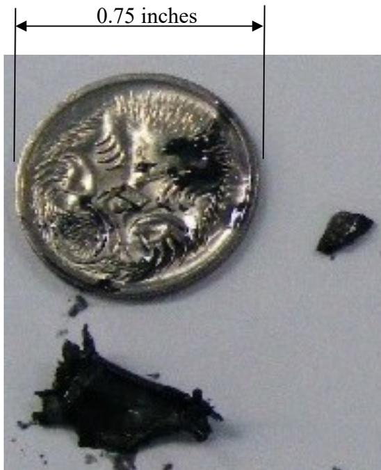
**RESULTS – CURRENT:** It has now been 18 months since the entire fleet was fitted with the OEI magnetic plugs. To date there has been no unscheduled failures of final drives resulting in increased dozer availability. The weekly plug inspection allows a proactive maintenance program by analyzing the trapped contamination and repairing the problem before it causes a serious failure and unscheduled downtime.
